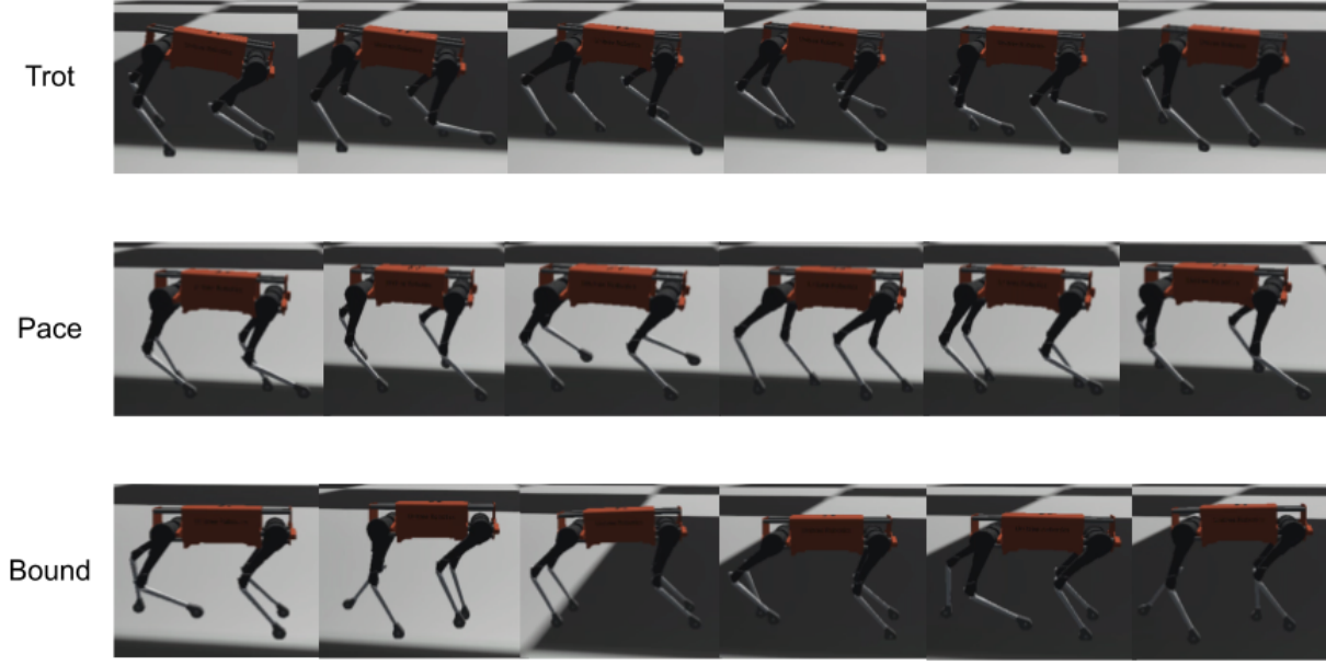
Fig. 3: Single gait learned using our hierarchical controller
