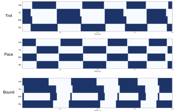
Fig. 7: Contact plot for each gait
