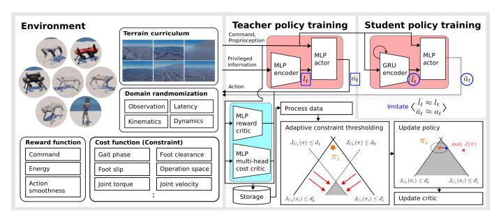
Fig. 2. Overall framework that leverages both rewards and constraints to train locomotion controllers for various legged robots
