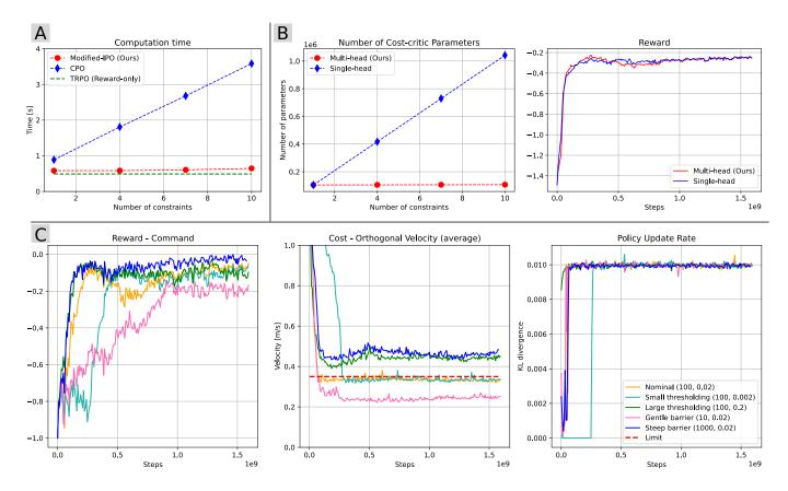
Fig. 6. Ablation study results of the proposed framework. (A) shows the computation time for different policy optimization algorithms. (B) shows the number of trainable parameters (left) and total rewards (right) for different cost-critic network designs. (C) shows the hyperparameter t and  $\alpha$  sensitivity in terms of the reward (left), cost (middle), and policy update rate (right).
