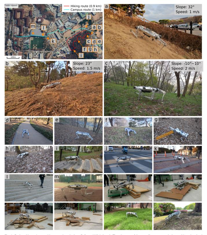
Fig. 4. Real-world experiments with two quadruped robots: Raibo and Mini-cheetah. The robustness of the controllers was extensively tested in various harsh terrains both indoor and outdoor. Outdoor experiments were conducted on two long paths: a hiking route and a campus route. The robot's speed is calculated using the video's recorded time stamp and the measured length of the traversal path. The slope of the environment is measured using a digital angle gauge.
